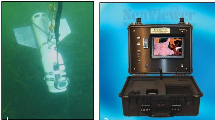
**Figure 6. Left: Seaviewer Camera. Right: Seaviewer Surface Unit and Recorder Interface**
