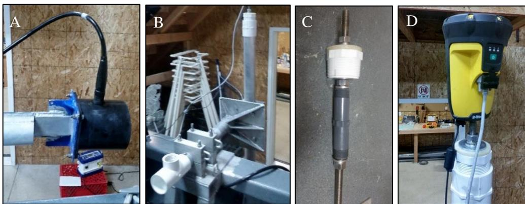
**Figure 5. A. Single Beam Sonar transducer with deck cable connected B. SBS mount in survey positions C. GPS mount. D. GPS with RS232 and micro USB cables attached**
