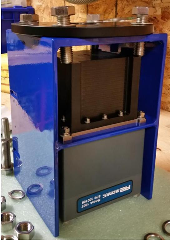
Figure 10. R2Sonic 2020 multibeam (bottom, grey), Applanix IMU (top, black), and mount (blue)
